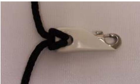
6. Measure down the rope to the next snap location and repeat these steps for the remaining flag snaps. If you are flying two flags allow about three inches between the flags.
